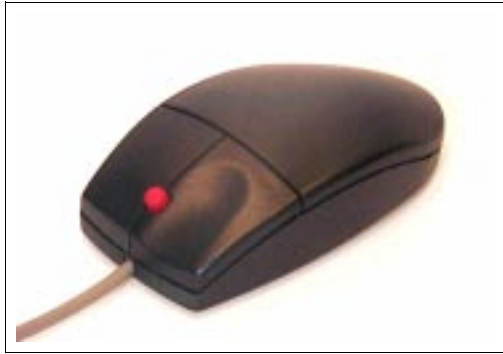
Figure 1 The Joystick Mouse is a mouse with an miniature joystick mounted between the two buttons.
